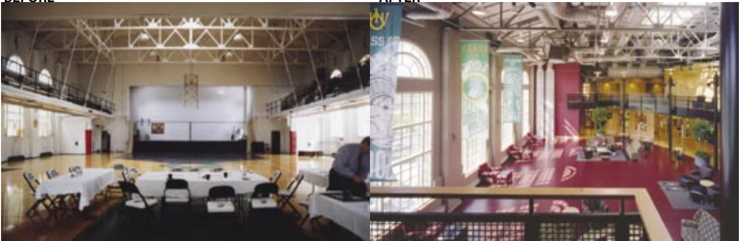
The flexible “living room,” Centre Court, can serve as a casual hangout space, formal function room, performance area or a venue for visiting speakers. The “before” image shows the first floor basketball court before the renovation. Existing bleacher stands seen in the “before” image were removed in favor of a new second story mezzanine.
