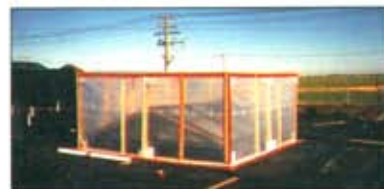
Figure 4: Chamber for pressurization/depressurization tests.
